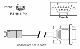
Figure A-3 RJ45 to DB-9 Adaptor
